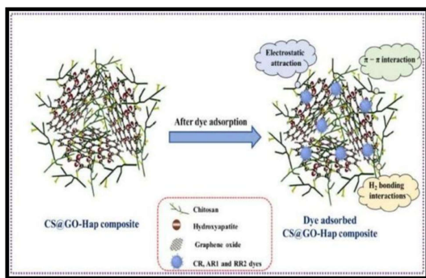
Figure 4: Dye removal by chitosan composites
