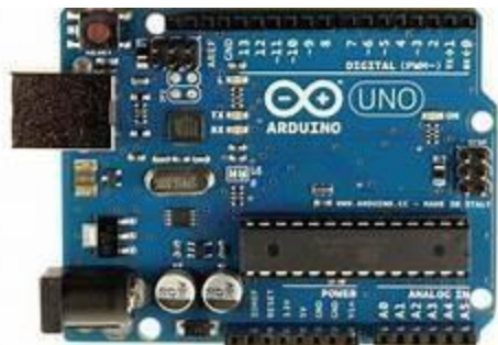
Figure 4 shows the Arduino microcontroller where the Arduino board can communicate at various baud rates. Baud measures how many times the hardware can send 0's and 1's in a second. The software used by the Arduino is Arduino IDE.
