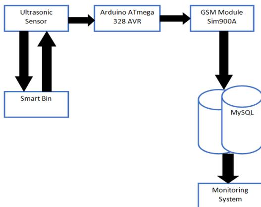
Fig 1 block diagram of waste monitoring system
