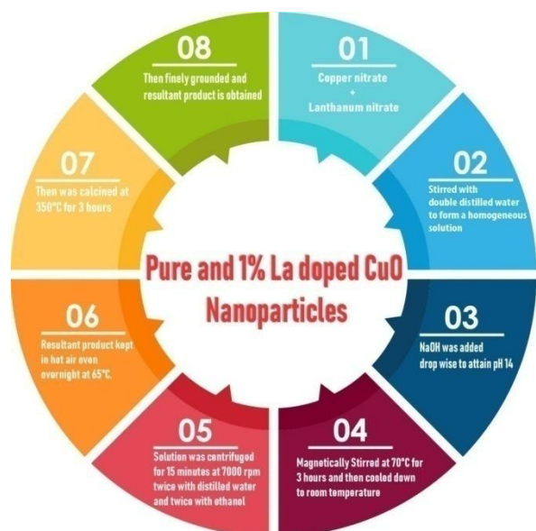
FIGURE 1: A schematic representation of synthesis procedure for pure and 1% La doped CuO nanoparticles
