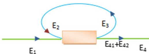
Fig.1 The diagram of single knot-shaped micro-nano-fiber system
