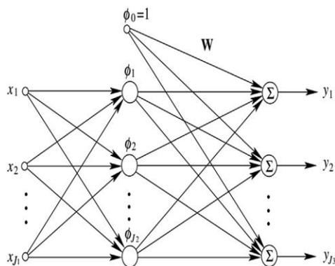
Figure 1 - Architecture of Radial Basis Function Neural Networks
