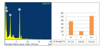
Fig.4. EDAX spectrum of Iron oxide nanoparticles
