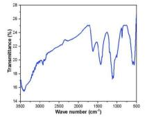
Fig.5. FTIR spectrum of Iron oxide nanaoparticles
