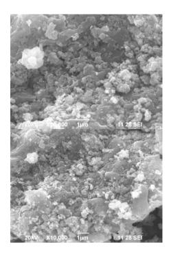
Fig.3. SEM micrograph of Iron oxide nanoparticles
