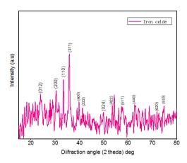
Fig.2. XRD patteren of Iron oxide nanoparticles
