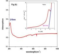
**Fig. 6(A).** UV–Vis absorption spectra of synthesized iron oxide nanoparticles, Fig B. Tauc's plots for the energy gap of iron oxide nanoparticle
