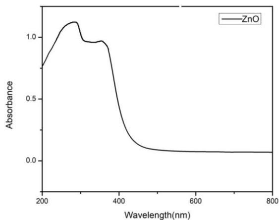
Fig 5. UV-Vis image of ZnO nanoparticles
