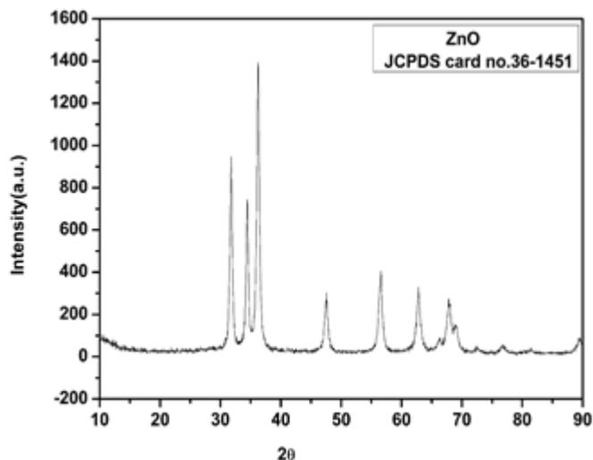
Fig 3. XRD image of ZnO nanoparticle.
