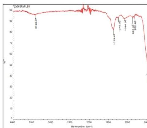
Fig 6. IR Spectrum of ZnO nanoparticles
