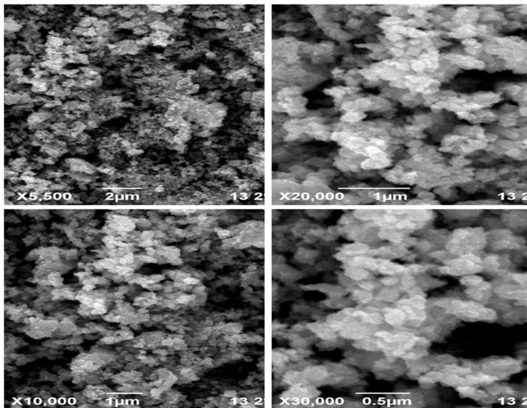
Fig 4. SEM-EDAX images of ZnO nanoparticles.
