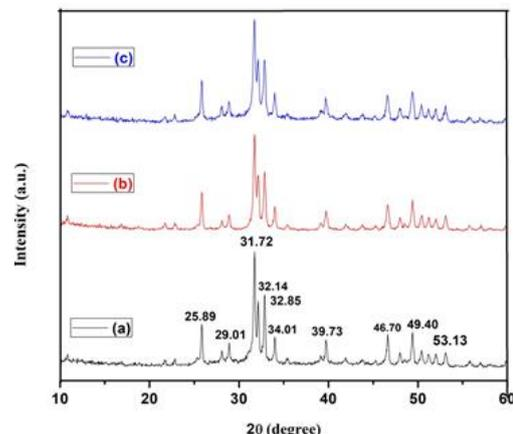
**Figure 2.** XRD spectrum of (a) HAP, (b) 0.1g Triton X 100 (c) 0.3g Triton X 100
