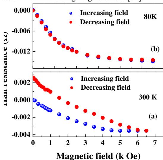
**Figure 5** Hall resistance curves at 300 K (a) and at 80 K (b) of Ni-Mn-Ga film grown at  $350^\circ\text{C}$
