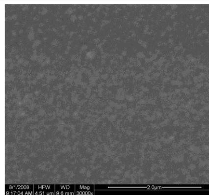
**Figure 2** SEM image of Ni-Mn-Ga film grown at 350°C
