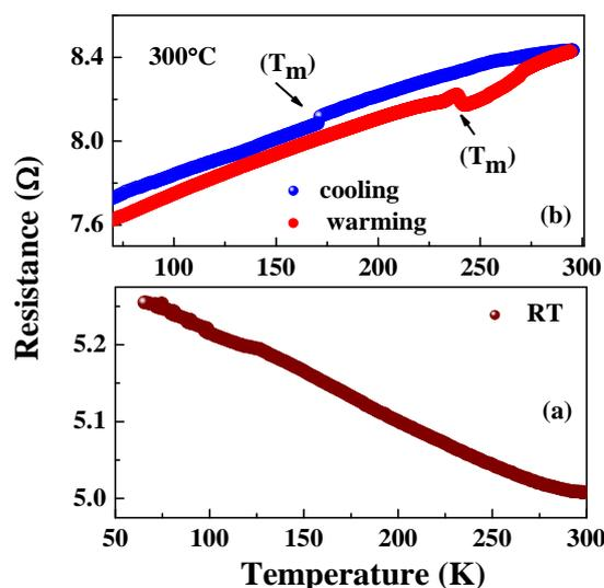
**Figure 3** Temperature variation of resistance of Ni-Mn-Ga film grown at RT (a); Temperature variation of resistance of Ni-Mn-Ga film grown at 350°C (b)
