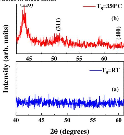
**Figure 1** XRD patterns of Ni-Mn-Ga film grown at RT (a); XRD patterns of Ni-Mn-Ga film grown at 350°C (b)
