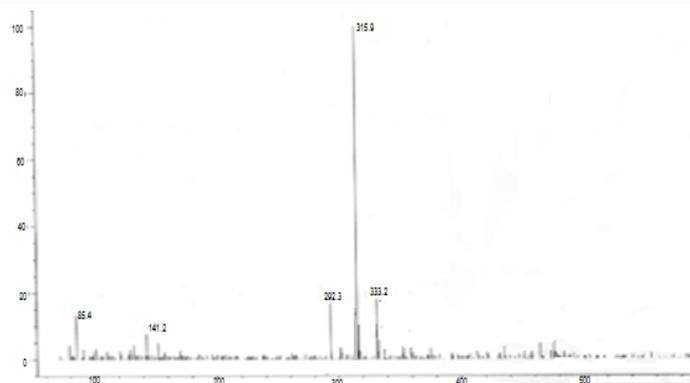
**Fig S3** Mass spectrum of EDHEAA
