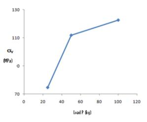
**Figure 6** Plot between load P and  $\sigma_{\nu}$
