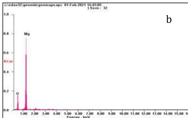
**Fig. 7. EDX pattern of MgO nanoparticles prepared in the presence of Orange Peel powder dried in a) Sun and b) Oven**
