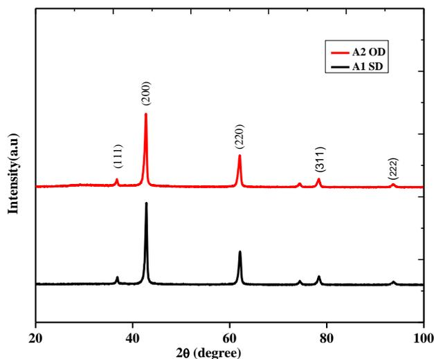
**Fig. 2. XRD pattern of MgO nanoparticles prepared in the presence of Orange Peel powder (A1) Sun Dried (SD) and (A2) Oven Dried (OD)**
