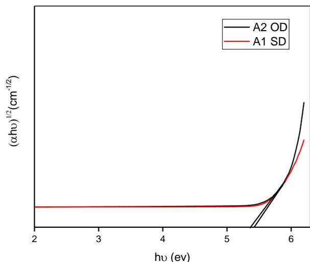
**Fig. 5. Tauc Plot of of MgO nanoparticles prepared in the presence of Orange Peel powder (A1) Sun Dried (SD) and (A2) Oven Dried (OD)**
