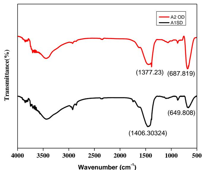
**Fig 3. FTIR Spectra of MgO nanoparticles prepared in the presence of Orange Peel powder (A1) Sun Dried (SD) and (A2) Oven Dried (OD)**
