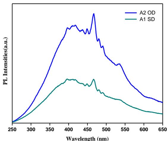
**Fig. 8. Photoluminescence analysis emission spectra of MgO nanoparticles**
