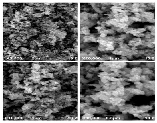
Fig 4. SEM-EDAX images of ZnO nanoparticles.
