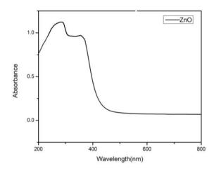
Fig 5. UV-Vis image of ZnO nanoparticles
