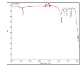
Fig 6. IR Spectrum of ZnO nanoparticles
