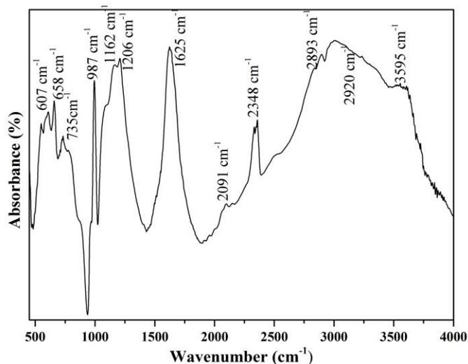
Fig.6 FTIR spectrum of grown Glycine Copper Sulphate single crystal
