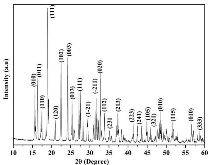
Fig.2 Powder XRD analysis of glycine copper sul
