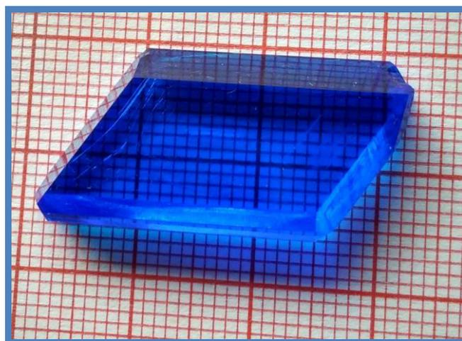
**Fig.1 Grown Glycine Copper Sulphate Single crystal**
