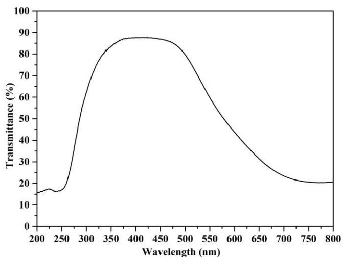
Fig.5 UV-Visible transmission study of grown glycine copper sulphate single crystal
