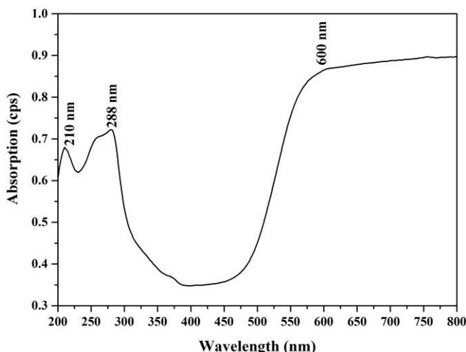
Fig.4 UV-Visible absorption study of Glycine copper sulphate crystal
