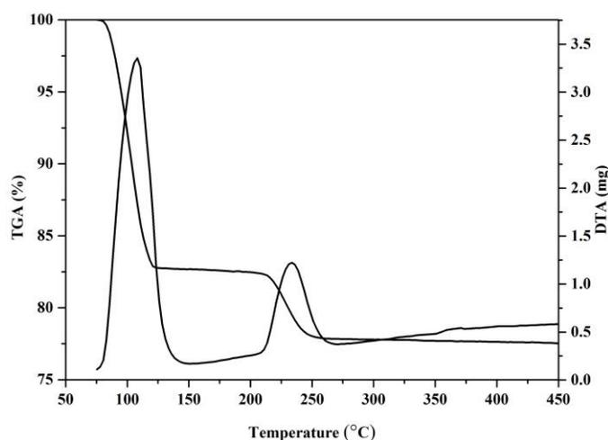
Fig.3 TGDTA curve of Glycine Copper Sulphate single crystal
