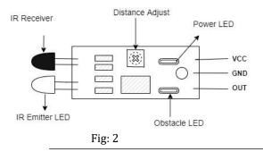
An IR (infrared) sensor is anmicroelectronicmodule that detects objects by detecting radiation from infrared emitted by them. It primarily consists of an IR LED transmitter and a photodiode receiver. It measures infrared radiation with wavelengths ranging from 700 nanometers to one millimeter.
