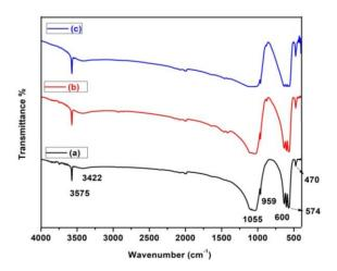
Figure 1. FTIR spectrum of (a) HAP (b) 0.1g Triton X 100 (c) 0.3g Triton X 100
