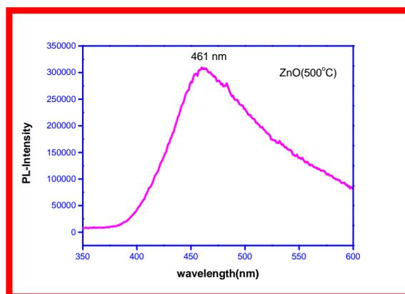
Fig.6. PL Emission spectra of ZnO NPs at 500°C
