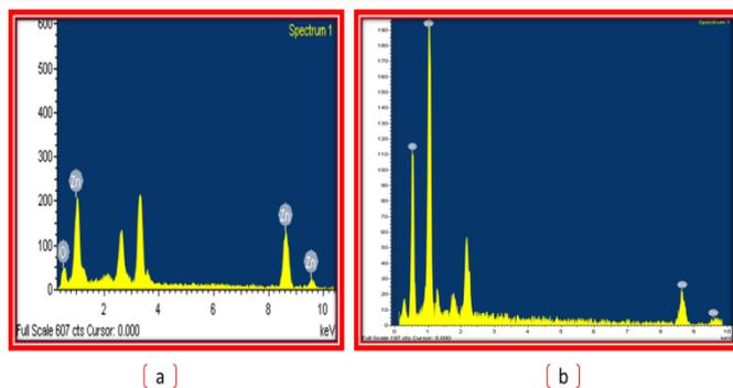
Fig.3. EDX spectrum of ZnO NPs (a) 400°C and (b) 500°C.
