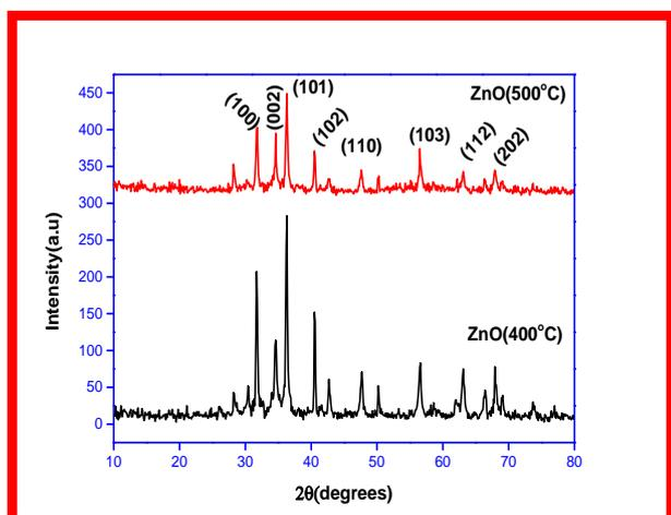
Fig. 1. PXRD pattern of ZnO NPs at 400 °C and 500 °C
