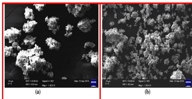
Fig.2. SEM image of ZnO NPs (a) 400 °C and (b) 500 °C.
