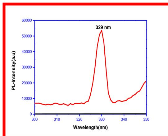
Fig.4. PL Excitation spectra of ZnO NPs
