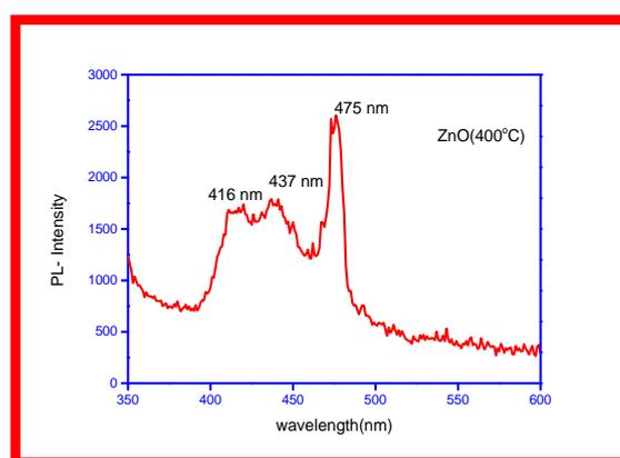
Fig.5. PL Emission spectra of ZnO NPs at 400°C
